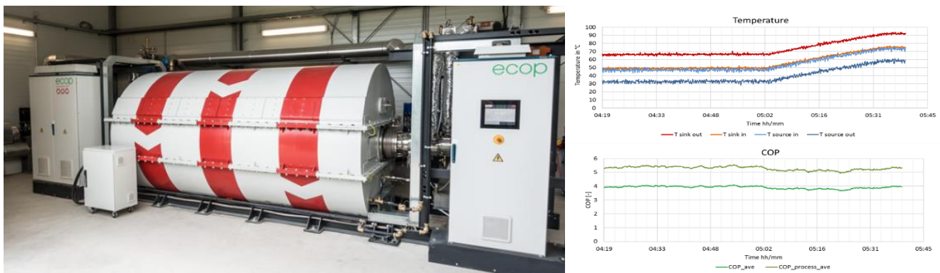
Figure 6: Reference system of a Rotation Heat Pump and test results based on Längauer et al. (2019)
