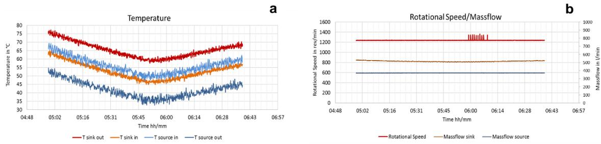
Figure 5: Temperature of sink and source (a), mass flow and rotational speed (b)
