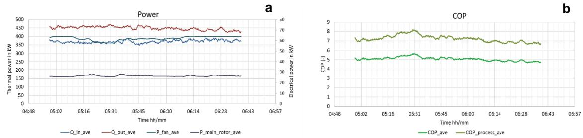
Figure 6: Thermal and electrical power (a), COP (b)
